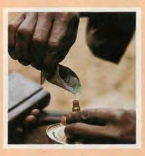
Leaf serves as powder funnel. Propellant is measured by eyeballing level against case neck.
